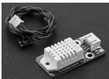
**Fig. 2: Temperature sensor**
